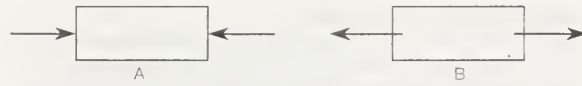
Figure 20: (A) Compression produced by equal and opposite forces. (B) Tension produced by equal and opposite forces.
